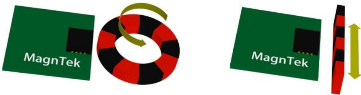
Figure-4: Off-Axis Applications with Magnetic Ring or Tape
